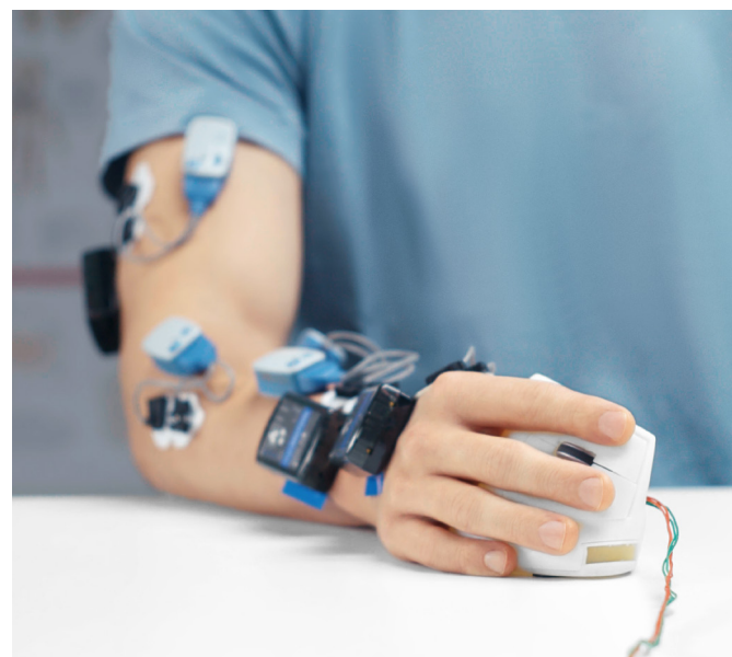
Logitech ergonomic testing with motion capture sensors
