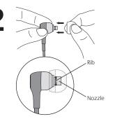
Attach ear cushions to earphone nozzle. Push ear cushion past rib on nozzle so ear cushion will not separate from nozzle during use.
