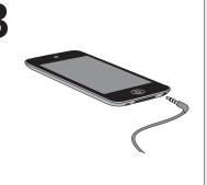
Insert the earphone cable connector into the 3.5 mm headphone jack on your iPod or MP3 player.
