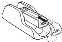
The headset LED shows the current charge status: red (low; <10%), yellow (medium; 10–<100%) or green when fully charged. Allow the headset to charge until it lights yellow or green before continuing (usually the headset ships with a partial charge).
