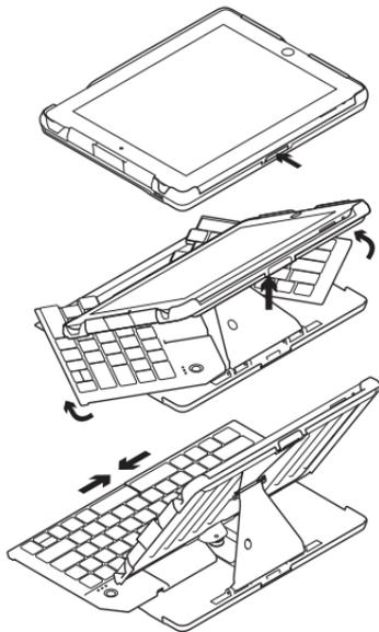
Press the release button and lift the iPad tray to expand the keyboard. The keyboard turns on when it is fully open.
