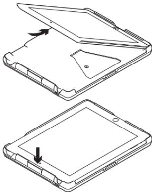
Slide your iPad 2 into the tray. Make sure that the connector port is aligned with the connector opening on the tray. Push the iPad into place. The “Click” lets you know that the iPad is securely attached.
