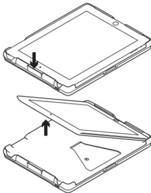
Press down on the iPad release to remove it from the tray.
