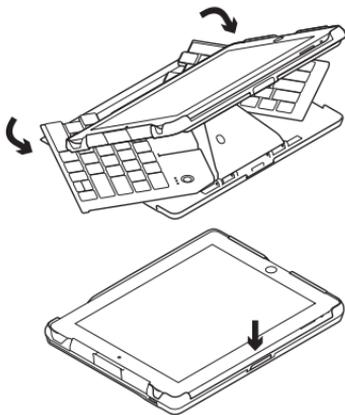
Hold and gently push both front corners of the keyboard towards the back of the unit until completely closed. Closing the unit turns off the keyboard.
