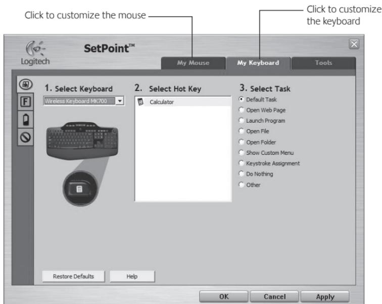
4. Choose a tab, such as the keyboard **F-key Settings**. A picture of the keyboard is displayed showing F-keys (list 2) to which tasks can be assigned (list 3).
