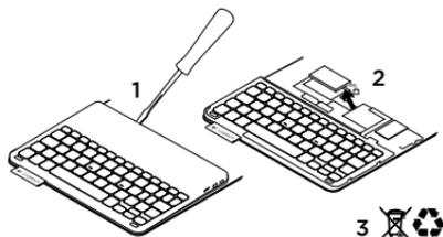
1. Pry off top cover of keyboard with screwdriver.
