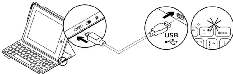
If the battery status light is red the keyboard folio battery needs to be charged.
