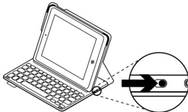
The Bluetooth light blinks to indicate that the keyboard is discoverable, ready for pairing with your iPad mini. The first time you turn on the keyboard it remains discoverable for 15 minutes.
