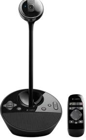
BYOD add-on solutions include microphone(s) and speaker(s) optimized for group situations that are used <u>in place of</u> the BYOD device's integrated mics and speakers. Note that some add-ons also include a video camera, and as a result provide both enhanced (group ready) audio and video functionality.
