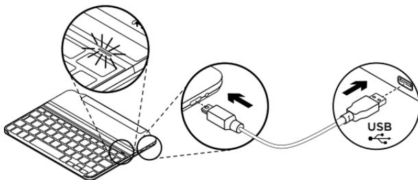
1. Plug one end of the micro-USB cable into the charging port, and the other end into a USB port on your computer.
