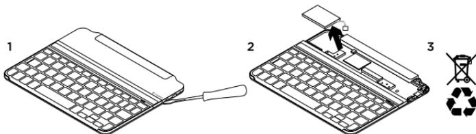
1. Pry off top cover of keyboard with screwdriver.
