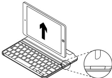
2. Push down: Apply downward pressure to ensure that the slot is completely flat:
