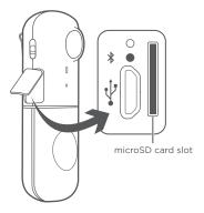
Your Bemo comes with a 4GB micro SD card preinstalled. The Micro USB port can be found on the side of the Bemo, below the *Bluetooth* pairing button.
