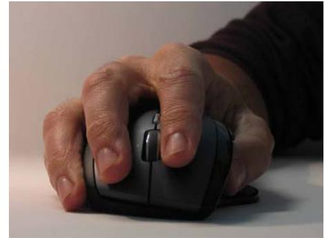
When a hand rests on the MX Revolution (shown above), it angles slightly toward a handshake position – a more comfortable, relaxed position. Below, the fingers and wrist are more level on a typical mouse, a position that requires more effort to maintain.
