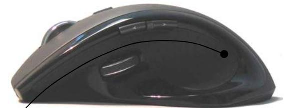
The arc length of the MX Revolution (shown above) – the distance from where the base of the typical index finger (second digit) and third finger rest to edge of the mouse keyplate – is 82 mm. According to a study of male U.S. Army personnel, the 90<sup>th</sup> percentile index finger length is approximately 81.6 mm. Also factoring in that the pad of the fingertip is approximately 8-10 mm from the fingertip, the MX Revolution provides more than enough length to support even very long fingers.
