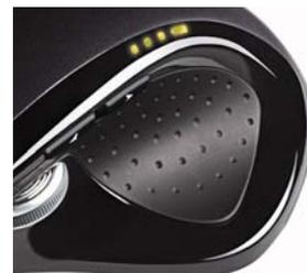
The MX Revolution mouse's dramatic thumb scoop provides support for the thumb. It also features a rubber grip pad and a sharp edge at the top that make it easier to pick up and move the mouse.
