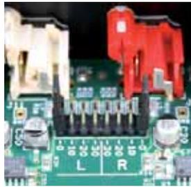
As it comes from the factory, Transporter is set for 0 dB attenuation. To adjust the attenuation, gently pull the black jumper conductors at the 0 dB position and move them to the position corresponding to the attenuation level you'd like. Choices include -10dB, -20dB and -30dB.
