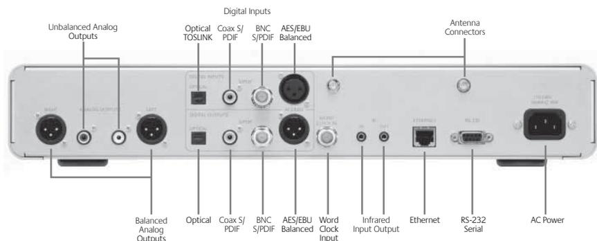
1. Connect an output from the Transporter to your stereo amplifier, preamp, or receiver with the appropriate interconnect.
