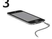
Insert the earphone cable connector into the 3.5 mm headphone jack on your iPod $^{\circ}$  or MP3 player.
