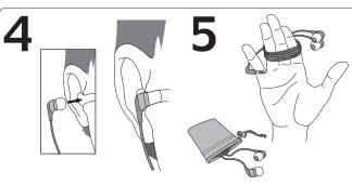
Gently insert earphone into your ear for a good seal: **R** for right ear; **L** for left. Never remove an earphone from your ear by pulling on its cable.
