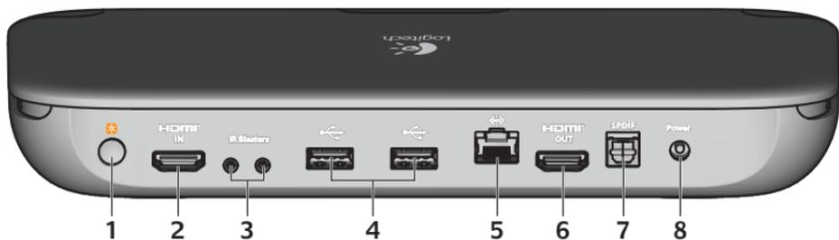
1. **Pair/Reset button** Use to pair the Keyboard Controller or other Logitech Unifying devices or to reset Revue to factory default settings.
