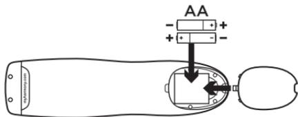
Insert the two AA batteries (included) into the battery compartment.
