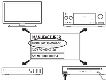
In order for Harmony 350 to control your entertainment system, we'll need to know the manufacturer and model number of each of the devices you own. The manufacturer and model number of your devices are typically printed on the front bezel, or on a label located on the bottom or the back of your entertainment devices. Write them down in the table provided on the back page of this Setup Guide for quick reference during setup.
