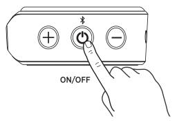
Note: To save power, X50 will automatically turn itself off after 15 minutes of no *Bluetooth* connection.
