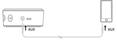
You can also connect X50 with any source devices using a 3.5mm auxiliary cable.
