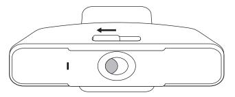
**3** To close the privacy shutter and cover the lens, move the slider to the right. The lens will appear white when the privacy shutter is closed.
