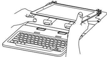
2 Lay the tablet holder flat and push the tablet upwards to release the bottom hooks from the tablet:
