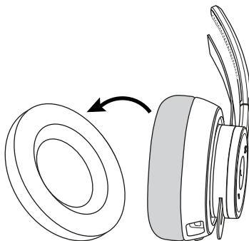
Make sure not to pinch the foam cushion which can be damaged easily.
