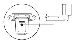
**2** Secure the webcam on your tripod by twisting it into the ¼ inch thread.
