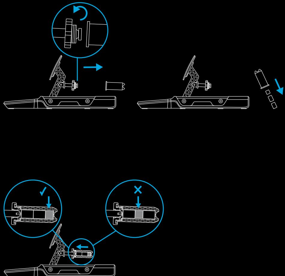
You can alter the feeling of the brake using the different pairings of elastomer pieces as determined by this table:
