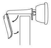
2 Adjust the webcam to make sure the end of the universal mounting clip is flush with the back of your device.
