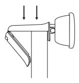
3 Manually tilt the webcam up or down to frame yourself within the camera's view.
