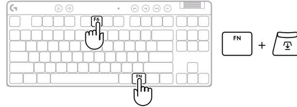
**3** Use arrow keys to increase or decrease the actuation point. You can also directly select the value you want by pressing the appropriate number (e.g. "4" for 1.5mm).
