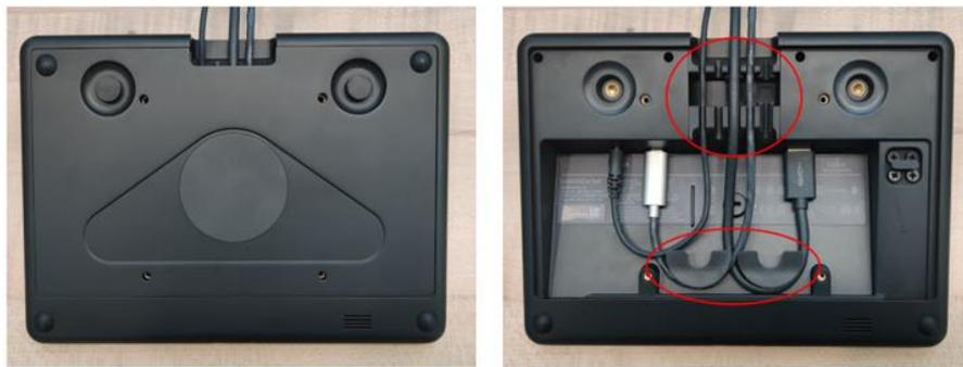
*Figure 6: Logitech Tap – Recessed Cable Well on the Back of the Device*
