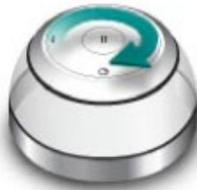
If you are not in CS2 application, gently gliding your finger clockwise or counter clockwise within the groove of the tooltuner dial will, by default increase or decrease system volume.
