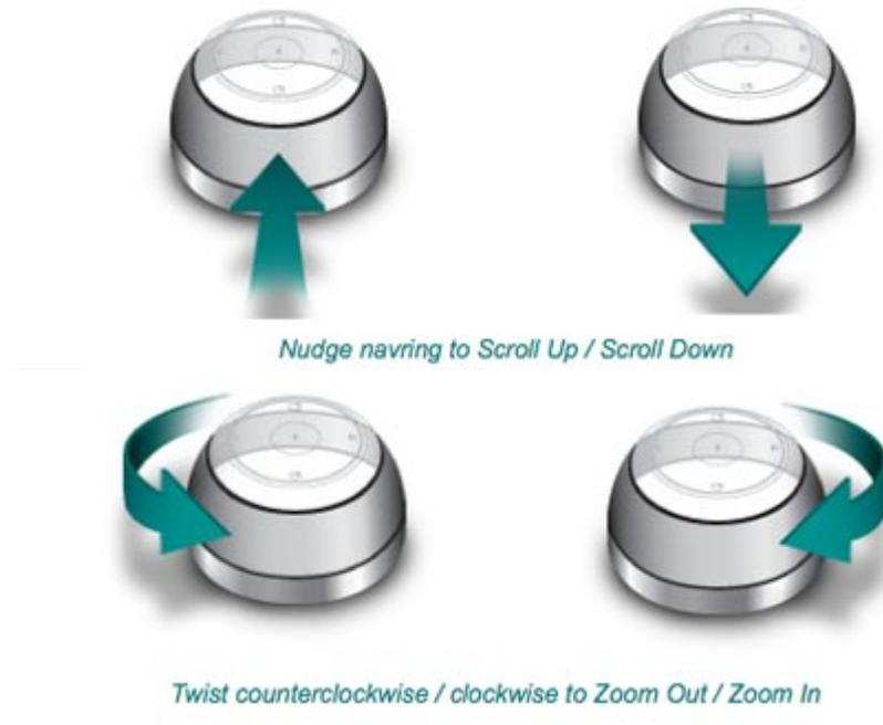
The navring also twists in a clockwise or counterclockwise direction. Twisting the navring will zoom in or out of images in the host application.
